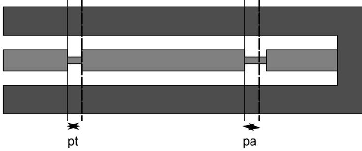
Figure 2: Ideal setup which can be achieved by using Kapton discs and specially shimmed test-ports to ensure the distance  $pt$ .
