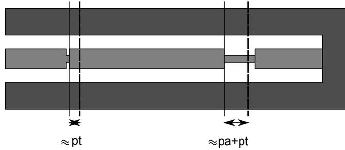
Figure 3: Result of mounting the air line without Kapton disk. The center conductor protrudes into the test-port.
