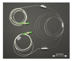
3: shows the practical realisation of an acetylene filled PC-HCF gas cell. The overall length of the fibre is a few meters. The very compact and flexible structure of the gas cell allows an easy implementation of such standards in measuring instruments.
