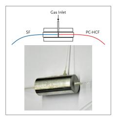
4: Gas tight connector adapter, principle and practical realisation.
