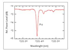
6: Doppler linear absorption of the P17 line of  ${}^{12}C_2H_2$ .
