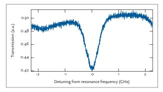
7: P16 line of  ${}^{13}\text{C}_2\text{H}_2$  as seen by tuning an AFTL source around the resonance frequency.
