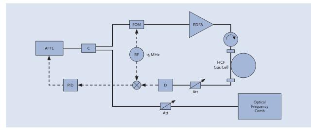
9: All-fibre optical setup for linear spectroscopy and laser stabilisation. AFTL: all-fiber tuneable laser; C: coupler; EOM: electro-optic modulator; EDFA: erbium-doped fiber amplifier; Att: attenuator; D: detector; PID: proportional-integral-derivative controller for laser lock. The Optical Frequency Comb allows to measure the frequency stability of the stabilised laser.
